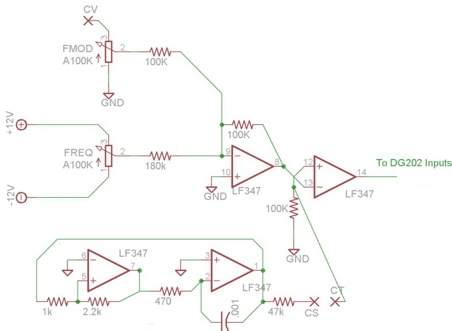
Above is the schematic for the frequency control. On the bottom left of the diagram is a triangle-wave oscillator created by combining a Schmitt trigger with an integrator. **NOTE FOR +/- 15v BUILDERS: Replace the 2.2k resistor with a 3.3k.** The output of this goes to the switch connector on the clock jack through a 47K resistor.
