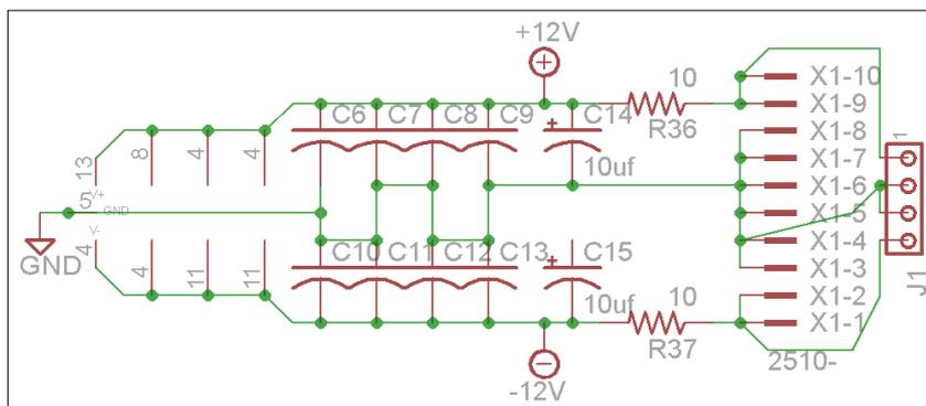
Above is the schematic for the power section. The positive and negative supplies are filtered with a 10 ohm and 10 uf capacitor, then the power pin of each IC has a .01uf capacitor near it to filter out high frequency noise.
