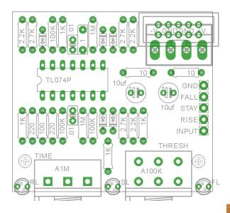
Wiring of this module is very straightforward. The tip connector of each jack should be wired to the corresponding wirepad. The GND wirepad should then be wired to the sleeve connector of one of the jacks.
