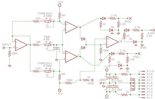
Above is the schematic for this module. On the left we see the main input connects to a 100K input impedance resistor and then onto an op-amp buffer. The buffer splits the signal three ways, at top and bottom it goes through 220 ohm resistors in series with the 100K dual gang Threshold pot. The threshold pot's two gangs form voltage dividers with the 1Meg resistors to +/-12V and the resulting
