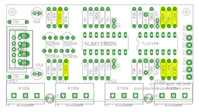
Above is a rendering of the PCB with the values shown for a 15V build instead of a 12V, the changed resistors are highlighted in yellow. These changes are untested, but should provide performance very close to the +/-12V version. The only other change that I wasn't sure about would be increasing the value of the 470K resistor at the emitter of the transistors, if the oscillator is reaching higher than useful frequencies you can increase the value of this resistor. The changes are:
