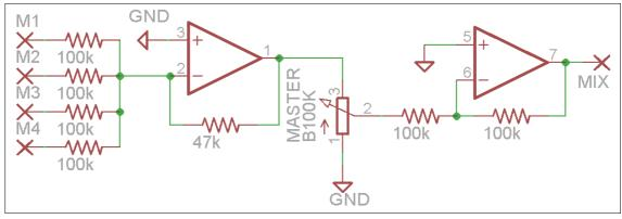
The mixer section just consists of an inverting gain stage that mixes the outputs, an attenuating potentiometer and a unity gain inverting stage.
