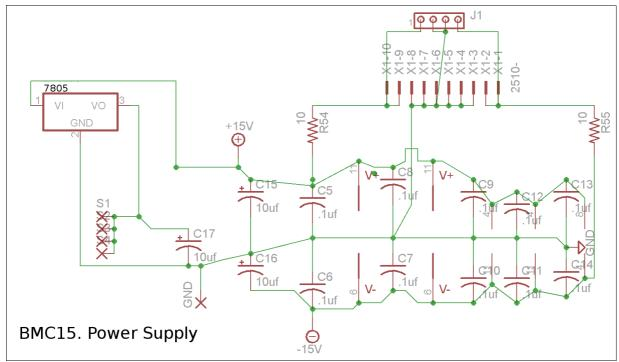
Finally we see the power supply. On the top are the power connecters. The 10 ohm resistors are used to filter out power supply noise. On the left is a 7805 voltage regulator, this is used to provide a steady 5v reference for normalizing to the CV attenuaters when no input is present. The rest of the schematic just shows the power rails connecting to the ICs supply pins and decoupling caps.
