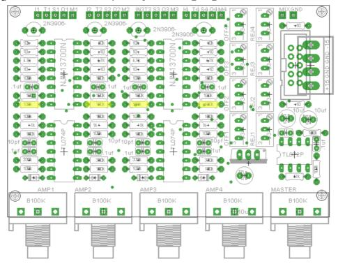
The board's dimensions are 3 and 5/8" by 2 and 3/8" (93mm x 62mm). The pots are spaced at 3/4" distance. The mounting holes are 3 1/2" x 2 1/8" (89mm x 53mm).
