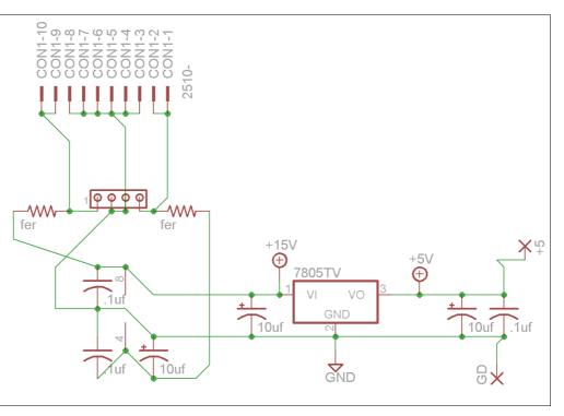
then filtered with another 10uf. There are additional .1uf caps for the power supply pins of each IC.
