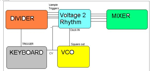
This patch gives a constantly shifting timbre. The keyboard's trigger output is sent to a divider's input, and it's outputs are sent to the V2R's sample trigger inputs. The keyboard's CV output is sent to the V2R's sample input, and a VCO's 1v/oct input. The square output of the VCO is sent to the clock input of the V2R. 4 of the outputs of the V2R are sent to a mixer. Each time a note is played on the keyboard, the V2R will resample one of it's outputs, and the clock's frequency will change.
