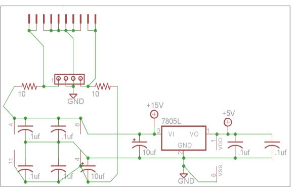
caps for the power supply pins of each IC.
