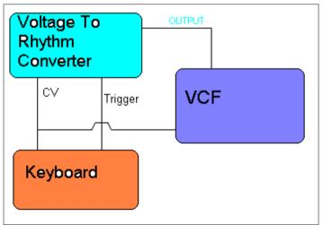
This is the first patch I ever did, when testing the original prototype. The VCF's Q should be cranked so that when the V2R's output is put into it's input, it produces a short, percussive sound. The V2R should be in trigger/series mode. With this patch, each note played will have it's own corresponding rhythm.
