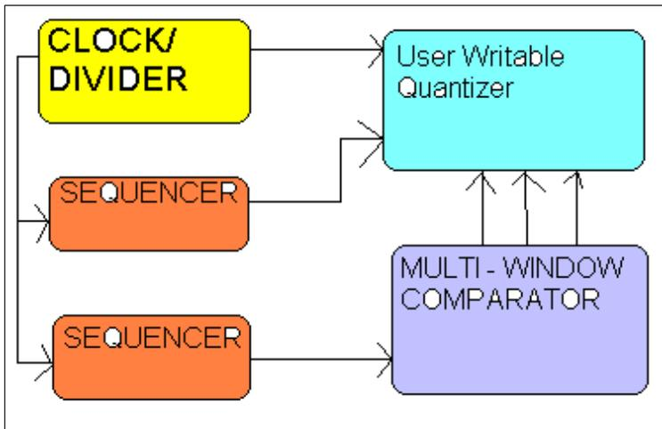
3. A Clock/Divider is sending outputs to the clock inputs of two sequencers and the trigger input of the UWQ. The first sequencer's CV out is going to the UWQ's CV in. The second sequencer's CV out is going to a Multi-Window Comparator's CV input. The gate outputs of the Multi Window Comparator are being sent to the Quantize input, the Aux CV in and the Aux Soft input. This patch will create a repeated series of notes that will sometimes be quantized, sometimes shift
