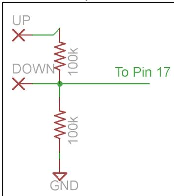
On the left, you see a schematic for the input for the UP/DOWN/BOTH switch. This is the same schematic as the Bank select switch. When 5V is applied to the UP terminal, it gets attenuated by the two 100k resistors and pin 17 sees ~2.5V. When 5v is applied to the DOWN terminal, pin 17 sees 5V.
