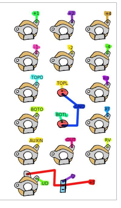
2. Advanced Wiring This version adds pushbuttons for all the *increase/decrease* step inputs and toggle switches which route the Reached Top and **Reached Bottom** outputs to the Reset and Reverse inputs. Diodes are added to act as passive OR type circuits to protect from shorts.
