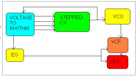
Stepped CV generator is then sent back to the Voltage To Rhythm converter to be used as it's input voltage. This creates a feedback loop where the Stepped CV's voltage output controls what trigger outputs the V2R outputs which in turn controls the Stepped CV's voltage output, etc etc. The Stepped CV's output is also controlling the pitch of a VCO.
