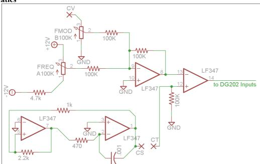
Above is the schematic for the frequency control. On the bottom left of the diagram is a triangle-wave oscillator created by combining a Schmitt trigger with an integrator. **NOTE FOR** +/-15v BUILDERS: Replace the 2.2k resistor with a 3.3k. The output of this goes to the switch connector on the clock jack.
