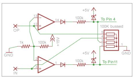
should turn on when any voltage higher than .1volts is inputted. On the comparator's output is a diode, 100K resistor and schottky diode followed by a 100K pulldown resistor. This network makes it so that the microcontroller only "sees" 0 and +5V, even though the comparator's output is actually +/-12V or +/-15V depending on your system.
