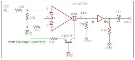
marked "OC." This VCA is incredibly simple, the signal is input to the inverting input through a 22K and 220 ohm resistor voltage divider used to limit the signal on the input. The output of the VCA goes through the onboard buffer and then a 10uf capacitor to decouple the DC bias.
