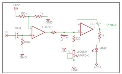
the wirepad marked "IN." A trigger or gate signal should be input here. The .01uf capacitor and 100K resistor to ground form a pulse shortener, making the pulse length of the input signal irrelevant. This is then input to an op-amp wired as a comparator. The output of the comparator goes to the decay section through a 1n4148 diode.
