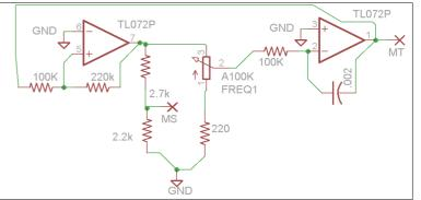
square wave output marked "MS" through a voltage divider (the schmitt trigger outputs +/-12V, these resistors attenuate it down to +/-5V). It then goes through a pot resisting the flow of current into the integrator, the 220 ohm resistor between the pot and ground sets the minimum frequency.
