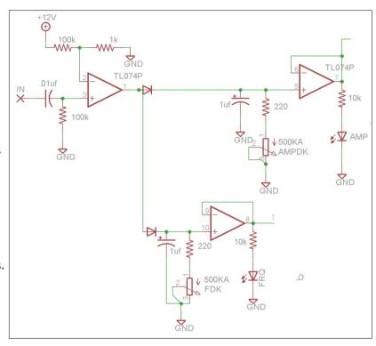
Each capacitor is also connected to an op-amp wired as a buffer, which is outputing the capacitor's voltage onto the next stage, as well as lighting up an LED indicator. The output of the Frequency Decay section goes to the VCO, and the output of the Amplitude Decay section goes to the VCA.
