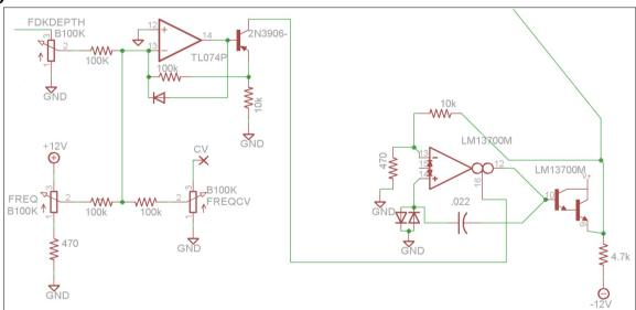
On the far left we see the input from the decay circuit. This voltage is summed with the voltages from the external frequency control and the baseline frequency control. These voltages are summed together on the negative input of the op amp wired in conjunction with a 2N3906 to form a linear voltage controlled current source.
