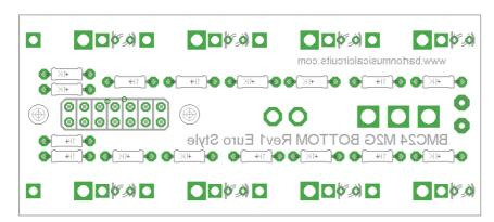
**STEP 11 -** *Stuff and solder the 1K resistors.* **STEP 12 -** *Stuff and solder the 14pin male header.*
