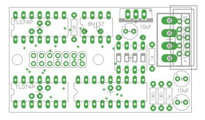
**STEP 5** - *Stuff and solder into place all the resistors. This includes a 10 ohm, 200 ohm, 1k ohm and a 100K ohm.*
