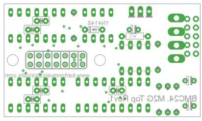
**STEP 1** - *Stuff and solder into place the 10 ohm resistor and the 1n4148 diode. Make sure the diode is oriented correctly, with the stripe pointing away from the resistor.*
