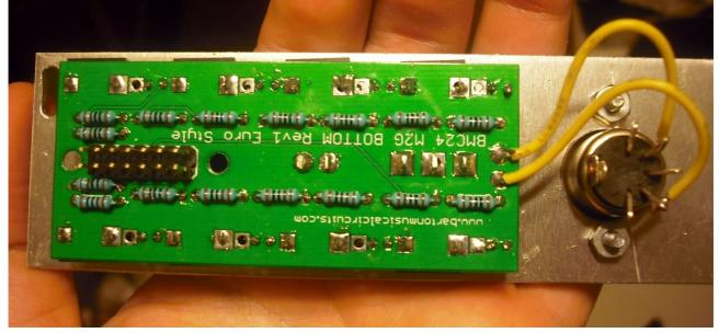
**STEP 25 -** *Connect the top PCB to the bottom PCB. If using standoffs, screw the top PCB to the standoffs.*
