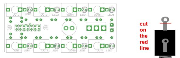
**STEP 13 -** *Prepare the 3.5mm jacks for stuffing. This means cutting the lugs off so they will fit in the PCB, like in the diagram to the right.*
